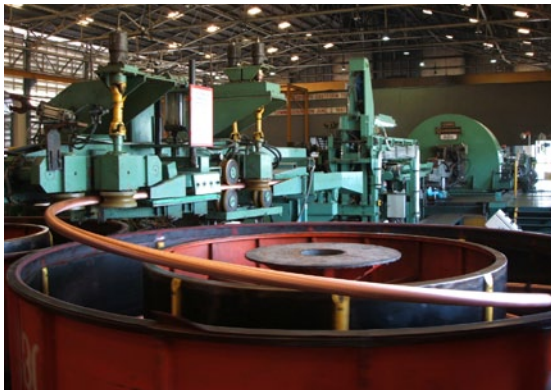
The planetary rolling mill at Luvata Hitachi Cable Thailand. The company is the fastest growing supplier of air conditioning (AC) installation tubes in Thailand
